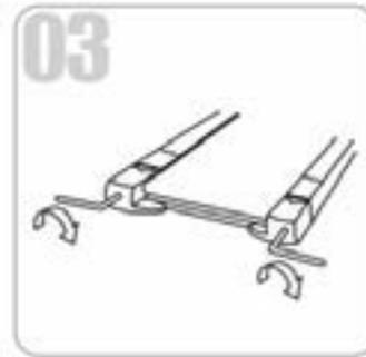
**(1) Running belt deviates to left** - Start the machine, set speed at 2-3 km/h without a load on the belt, use Allen key to turn the screw 1/4 turn (see fig. 1). Then allow the machine to run without a load for 1-2 minutes. Repeat process until the belt becomes central.
