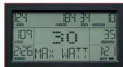
Maximum watts produced during all strokes
