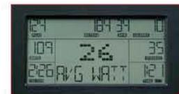
Average watts per stroke based on all strokes
