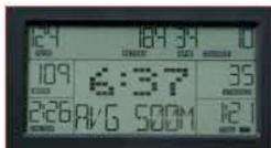
Projected time needed to complete 500 meters based on all strokes
