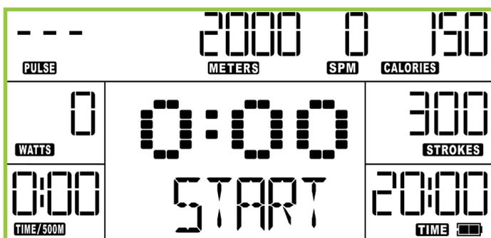
1. During the program, the TIME, STROKES, CALORIES, and METERS displays will count down to zero and will stop at zero.
