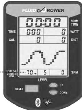
The Monitor will automatically pair with the nearest Bluetooth heart rate device. When pairing is complete, the Monitor will jump back to the initial screen and begin to display the heart rate.
